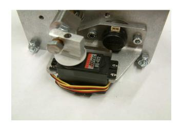
Step 4: Using four 8-32 x  $^{1}/_{2}$ " screws, mount the servo onto the bracket.
