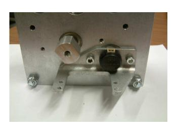
Step 2: Screw the servo post assembly into the shift block. Use a  $^{7}/_{16}$  wrench to tighten the servo post assembly while holding the shift block with the  $^{5}/_{8}$  wrench.
